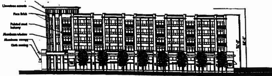
South Building -Cicero Ave. Elevation
