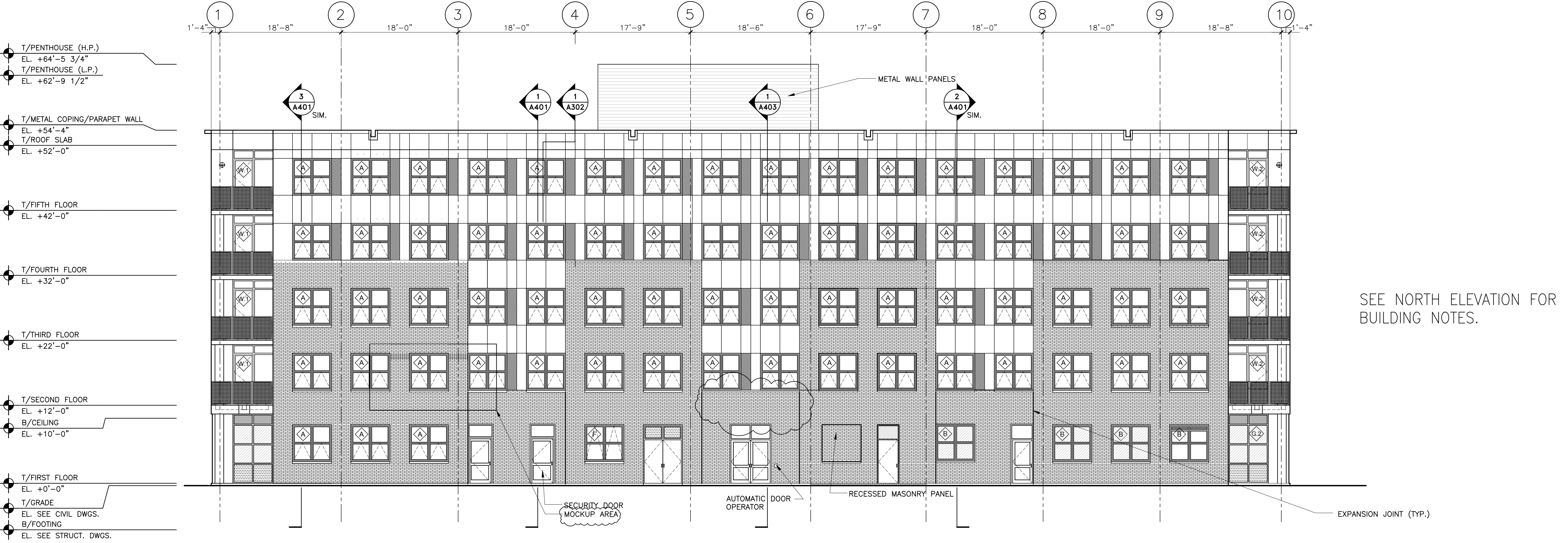
2 NORTH MIDRISE - SOUTH ELEVATION - (ALLEY ELEVATION) SCALE: 1/8"=1'-0"
