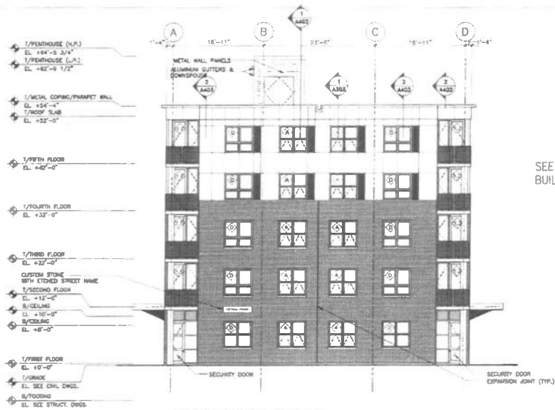
1 WEST ELEVATION—(FEDERAL STREET ELEVATION) SCALE: 1/8"=1'-0"
