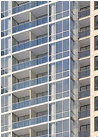
Lighter Facade : Facade is articulated with a higher percentage of glazing with a contrasting color at slab edges and verticals
