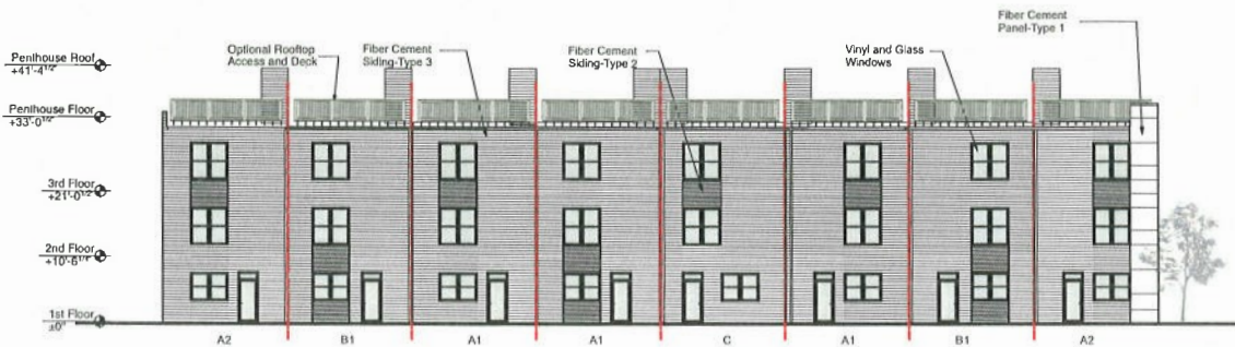
East Elevation - Building 1
