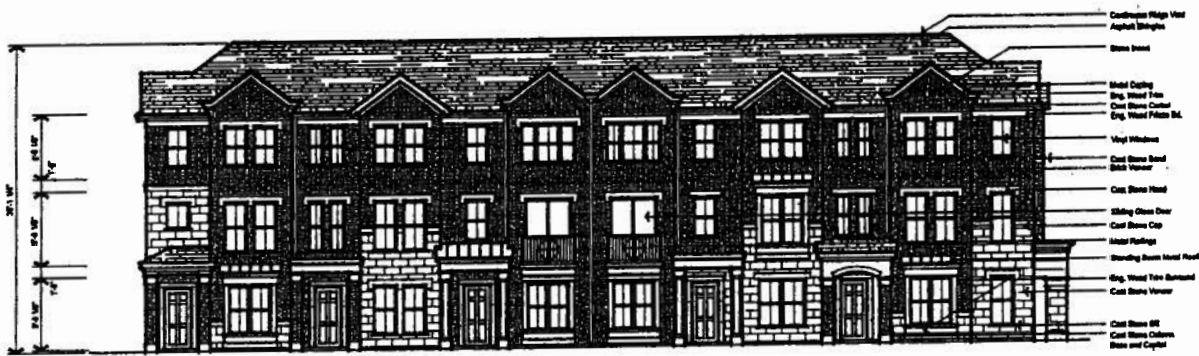
Front Elevation Typ. 6 Unit Bldg. 3/16" = 1'-0"
