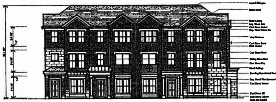
Front Elevation Typ. 4 Unit Bldg. 3/16" = 1'-0"
