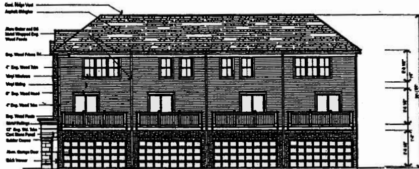
Rear Elevation Typ. 4 Unit Bldg. 3/16" = 1'-0"
