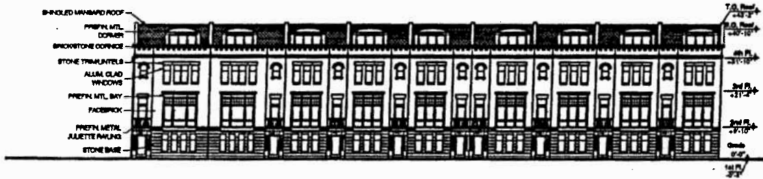
Front Elevation (Interior Drive)
