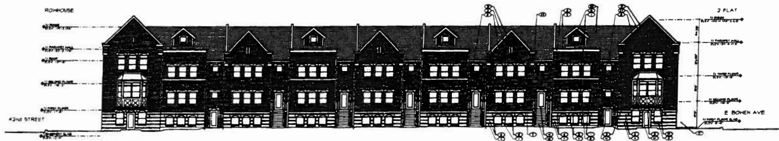
PARCEL B-DREXEL BLVD. ELEVATION SCALE 1/4" = 1'-0" ROOF ELEVATION OF THE BRICK FAMILY WITH FLATS ON THE ROOF
