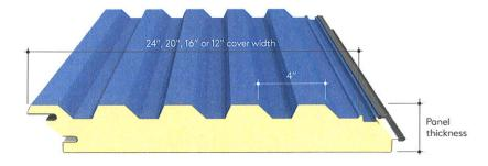
Designwall R Series, a profiled, accent version of BENCHMARK Designwall 2000 with ribs at <sup>7</sup>/8" deep. The asymmetrical profile is designed for horizontal or vertical application. The R Series panel adds a bold, profiled look to commercial construction. Designwall R Series interfaces and engages with other Designwall horizontal panel profiles.
