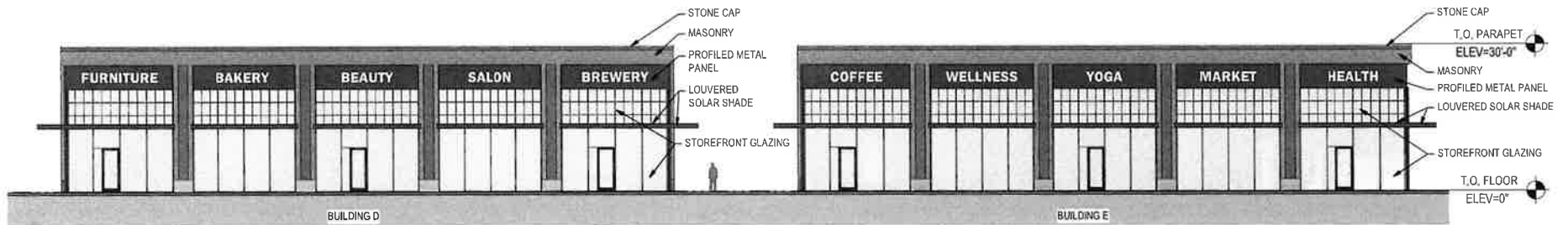
2 BUILDINGS D&E - SW ELEVATION
