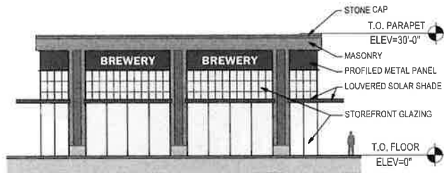
4 BUILDING D - SE ELEVATION
