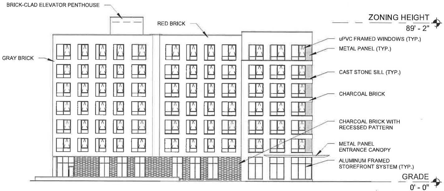
1 WEST BLDG - SOUTH ELEVATION 1/32" = 1'-0"
