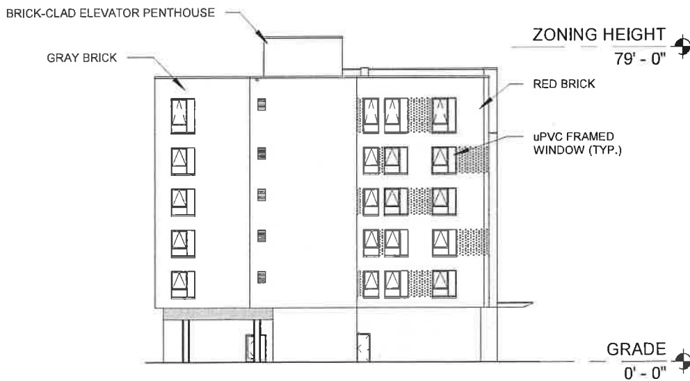
1 EAST BLDG - NORTH ELEVATION 1/32" = 1'-0"
