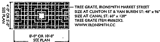
3 TREE GRATE PLAN SCALE: NOT TO SCALE
