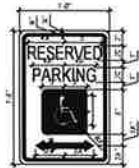
R7-8 HANDICAPPED PARKING SIGN N.T.S.
