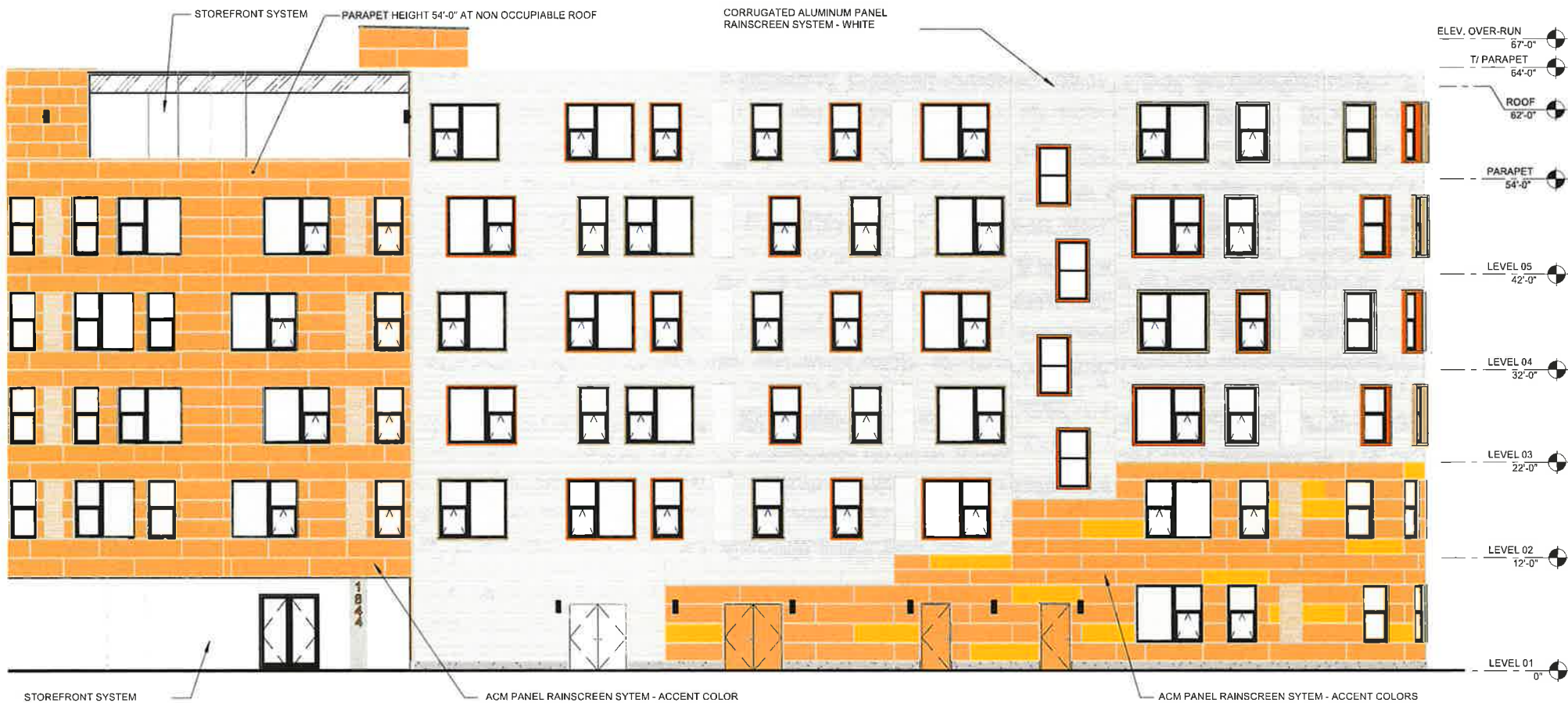
1 EXTERIOR ELEVATION - EAST 1" = 10'-0"
