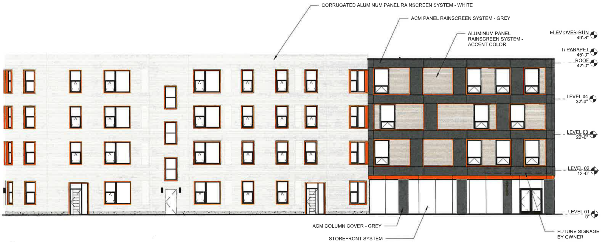
1 EXTERIOR ELEVATION - NORTH 1" = 10'-0"
