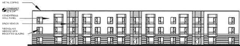
BUILDING D1 MULTI-UNIT RESIDENTIAL WEST ELEVATION
