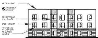
BUILDING D2 MULTI-UNIT RESIDENTIAL SOUTH ELEVATION
