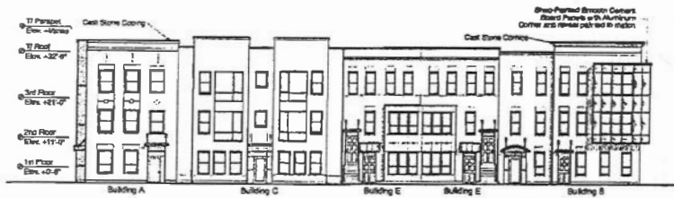
West Elevation C - Evans Ave. (Group F) SCALE: 1" = 30' Note: This building design is tentative as pertains to Phase II construction.
