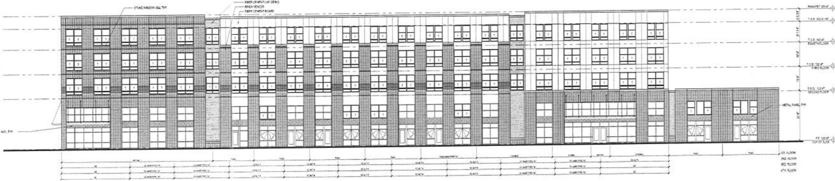
1 BUILDING I - WEST ELEVATION SCALE: 3/32" = 1'-0"
