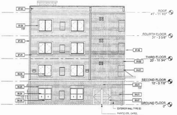
② 02 - EAST - ELEVATION 1/8" = 1'-0" BUILDING 01, 02, BUILDING 03, SIMILAR.
