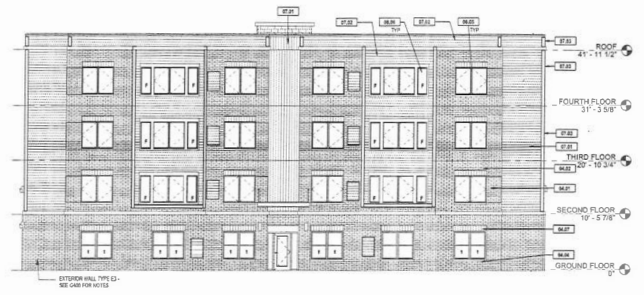
① 01 - NORTH - ELEVATION 1/8" = 1'-0" BUILDING 01, 02, BUILDING 03, SIMILAR.
